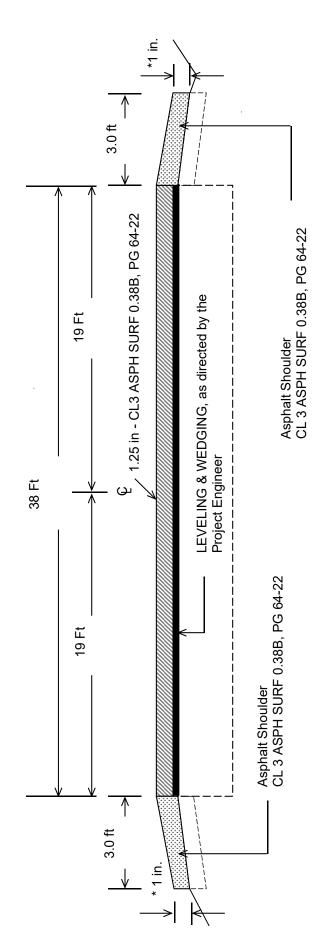
Asphalt Milling & Texturing Overall Average Depth 1.25" Width of Milling 44 FT
